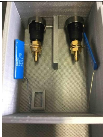
Bolting of 10 M \Omega resistors onto the sockets
